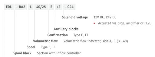
**Basic type** Type EDL: directly actuated proportional directional spool valve
